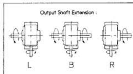
To order indicate Model, Output Shaft Extension and Ratio, as shown below
